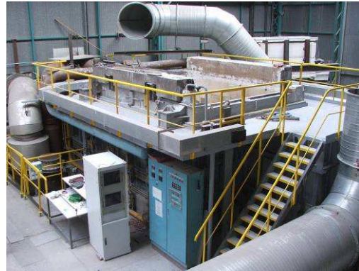
Fig. 2 ISO 834 and HCM curves and global view of the gas-burners furnace
