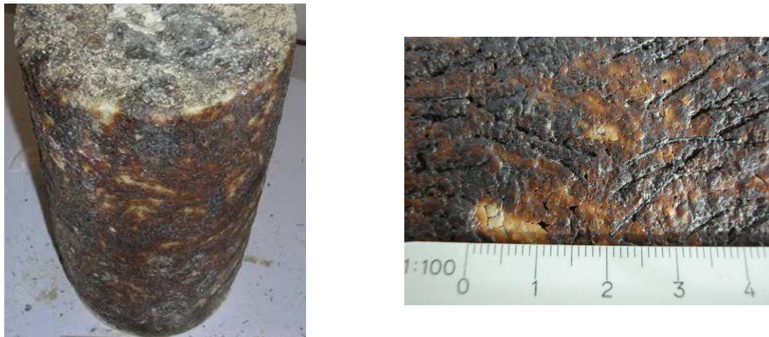
Fig. 10 On the left, global view of a sample after HCM test. On the right, zoom on the sample surface
